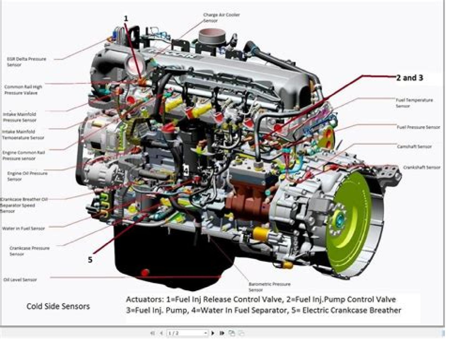
Actuators: 1=Fuel Inj Release Control Valve, 2=Fuel Inj. Pump Control Valve
