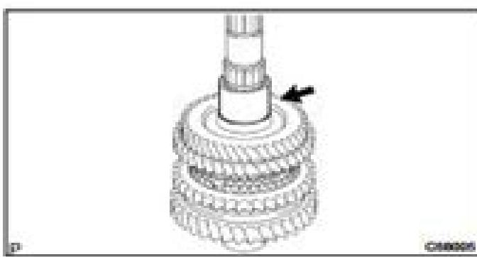
**6. REMOVE OUTPUT GEAR SPACER**
